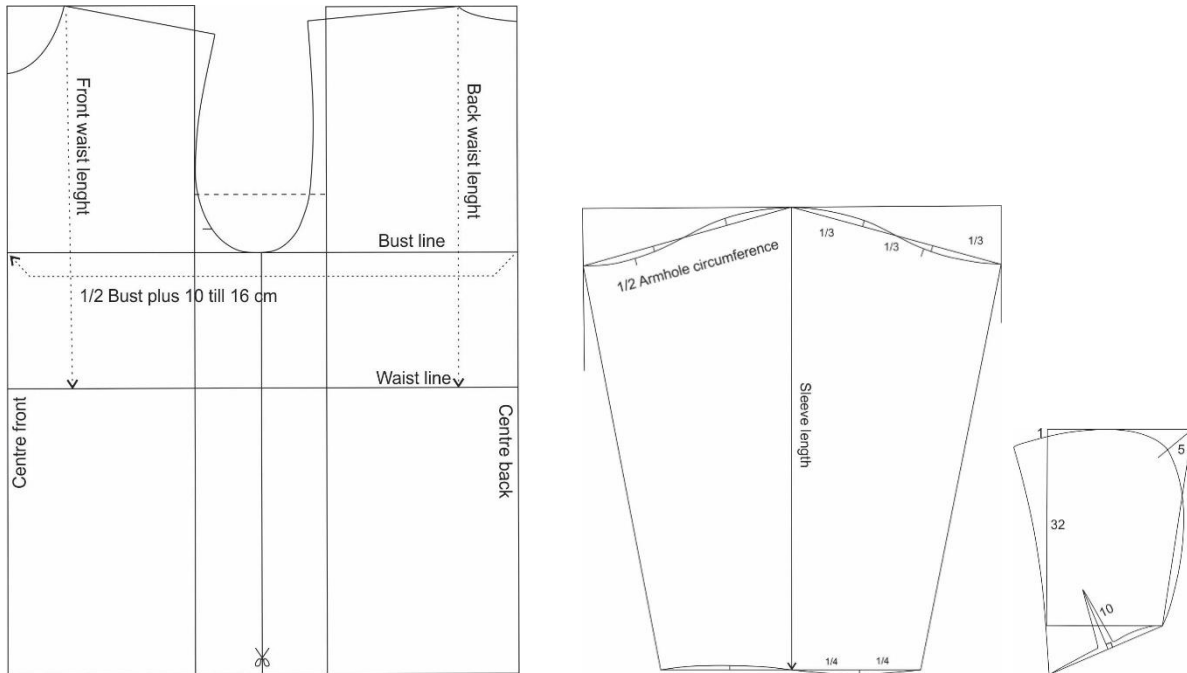
Figure 3: Basic block pattern of men's shirt: front and back part, sleeve and hood (Ujević et al., 2000, Jansen and Rüdiger, 1990)
