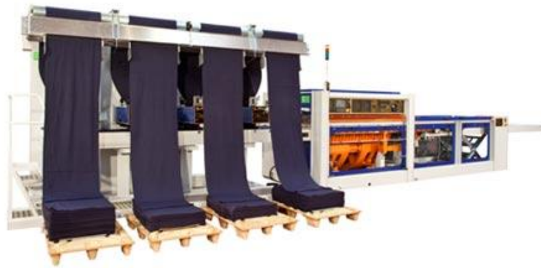
Figure 6. Automated cutting system for tubular fabrics AC3 developed by company Bierrebi
